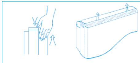
2. Remove the inner front panel by unscrewing the screws along its top and sides. As the front insulation is attached care must be taken when lifting this panel from the heater and placing it to one side.
