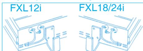
7. Place the heater on its feet, and in the desired position against the wall - **DO NOT LIFT THE HEATER BY ITS TOP PANEL!** Ensure that the heater is based on a firm level surface, at least 100mm from any end wall, and at least 100mm below any shelf or similar projection. Cut away the gripper rod or carpet which would prevent the heater sitting firmly on the floor.
