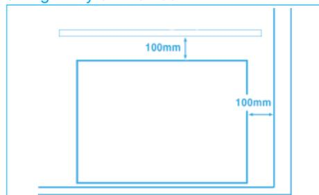
8. Mark the position of the two outside corners of the wall bracket with the heater pushed tight against the wall. Remove the wall bracket from the heater by removing the screw at each end. Place the heater to one side and reposition the bracket against the wall using the corner marks for alignment.
