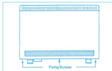
14. Finally, tighten the screws at each end of the wall bracket. Ensure that all screws have been tightened as this is essential to maintain earth continuity.
