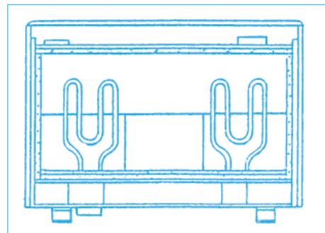
12. Fit the front layer of bricks with the recess toward the front of the heater.
