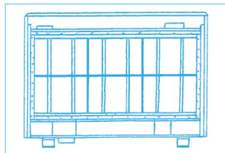
13. Replace the inner front, complete with insulation, by locating its bottom edge behind the front lip of the chassis and inserting the retaining screws along the top and sides.
